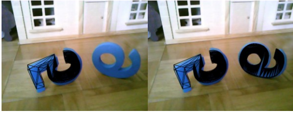
Figure 4. Result of pose estimation of a single object “5” (left) and multiple objects (right).
