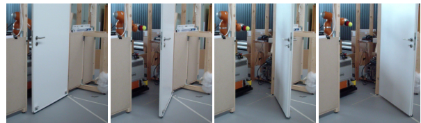
(a) Being able to predict the dynamic behavior of the door, the robot can swing it open precisely to a desired state, here 60^\circ . The manipulation time from touch to release of the door is approximately one second.
