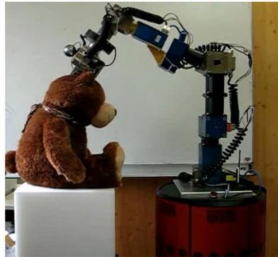
Fig. 1: Our mobile manipulation robot Zora.
